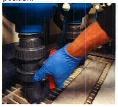
Turn the blue pressure release valve from horizontal closed position to vertical open position at the bottom of the canister to drain the residual water out of the canister filter.
