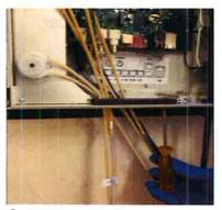
Disconnect the dosing head in need of repair by simultaneously pressing the side latches and carefully pulling the head off of the motor rod, then disconnect the lines leading to the dosing head.
